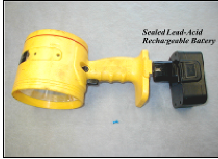
Prohibited: Rechargeable sealed lead-acid battery commingled with other scrap
